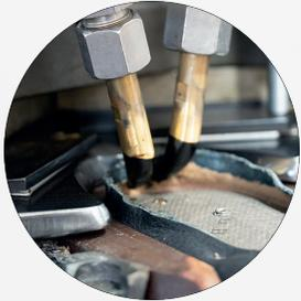
Thermocement application by tracers directly on the insole
