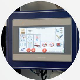
7" Touch screen programming system with styles storage on USB key, autodiagnostic functions
