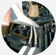
Total thermocement application by two movable tracers suitable for any kind of shoe in any size
