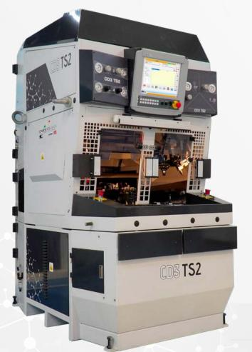
With two independent heads to apply two different kind of cement (e.g. primer + cement) on the same shoe, or the same cement for high productivity working.
