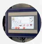
7" Touch screen programming system with styles storage on USB key, autodiagnostic functions
