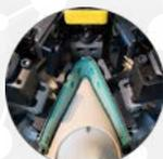
Teflon with 5 pressure points, quick change, vertical upper presser with programmed pressures
