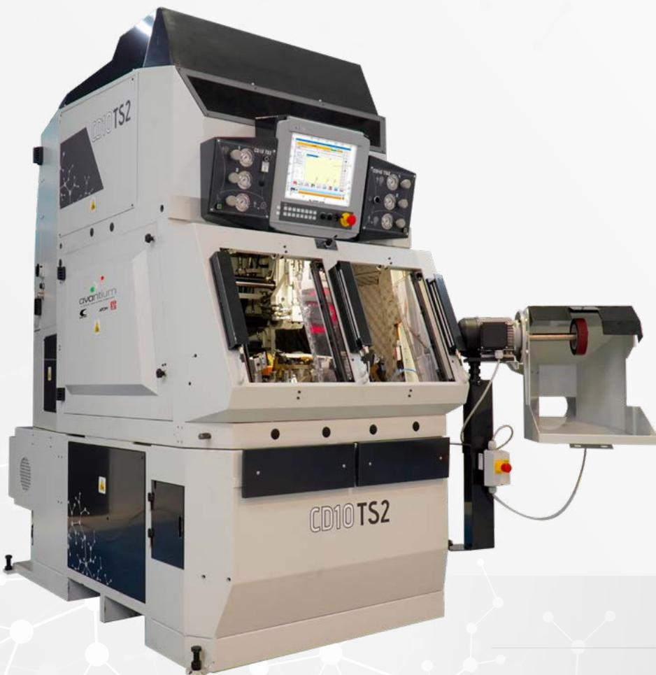
With two independent heads that carry out the operations simultaneously. Alternately, both the heads can be set as rough-milling/rough-milling or roughing/roughing for high productivity working.
