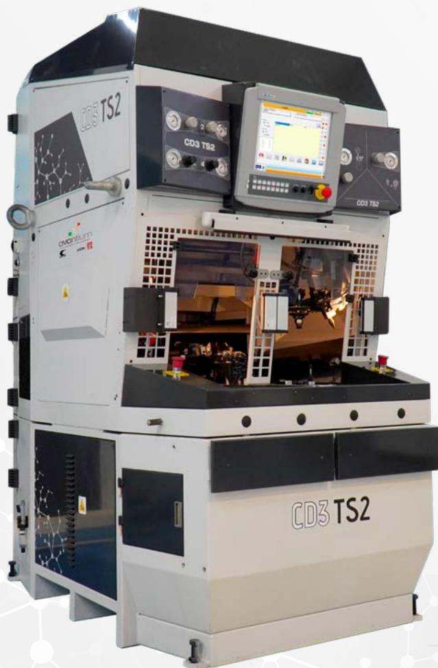
With two independent heads to apply two different kind of cement (e.g. primer + cement) on the same shoe, or the same cement for high productivity working.
