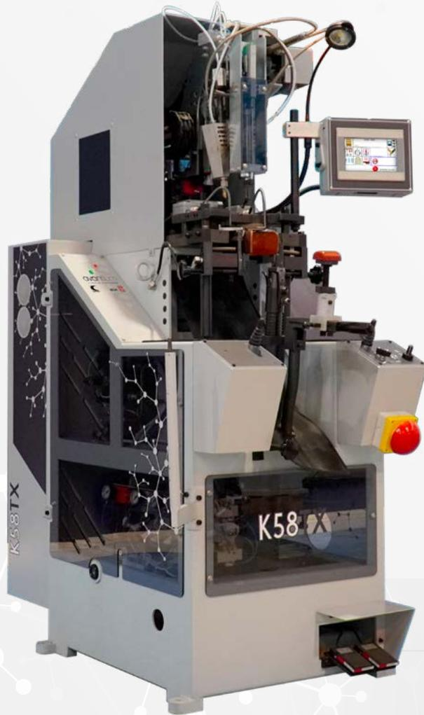
The K58TX born on the natural evolution of the well known K58STI. The cement is applied by tracers directly on the insole.
