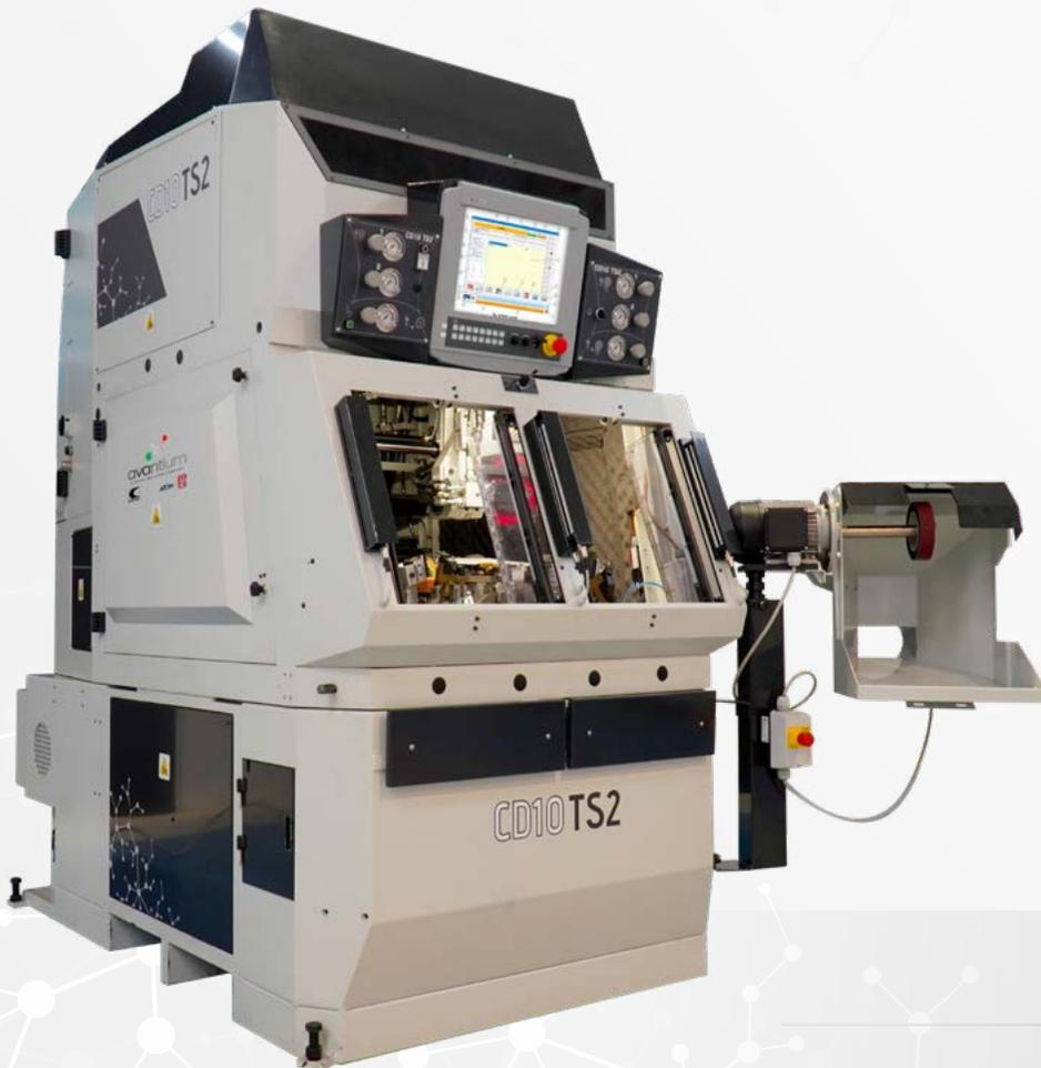
Pounding/roughing o rough-milling/pounding machine for the shoe bottom, with two independent heads that carry out the operations simultaneously.
